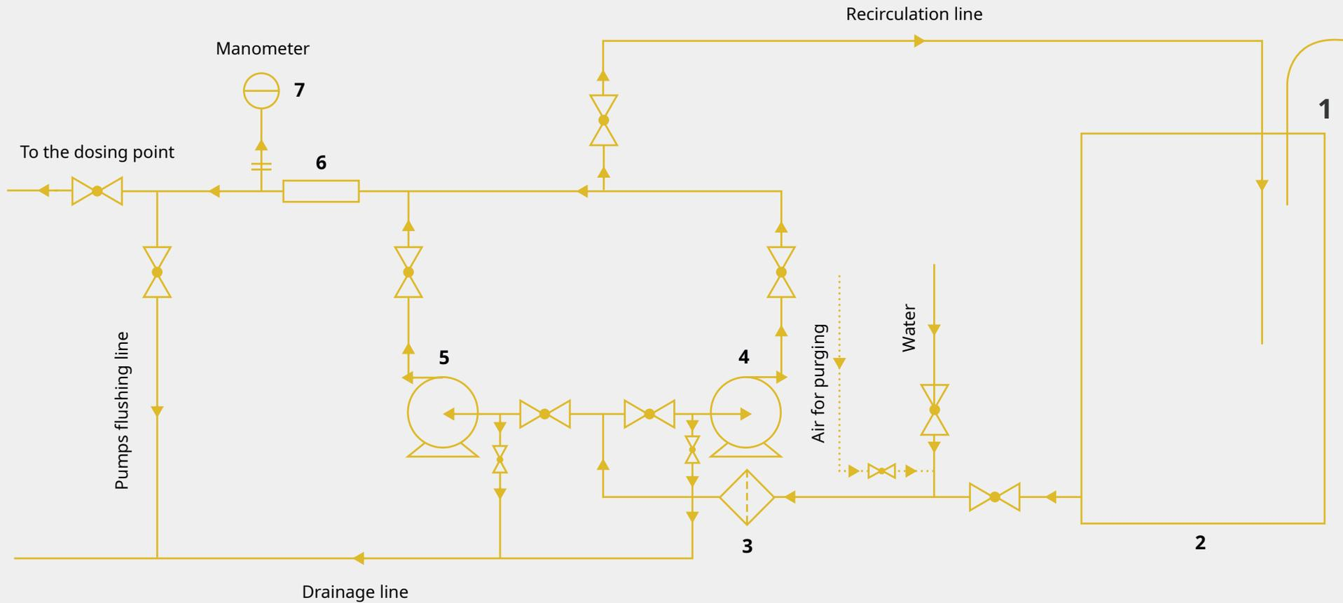
1 — ventilation; 2 — reservoir for suspension storage; 3 — mesh filter; 4 — main dosing pump; 5 — reserved dosing pump; 6 — area from transparent material (polycarbonate); 7 — manometer for detection of working pressure and possible leakages
