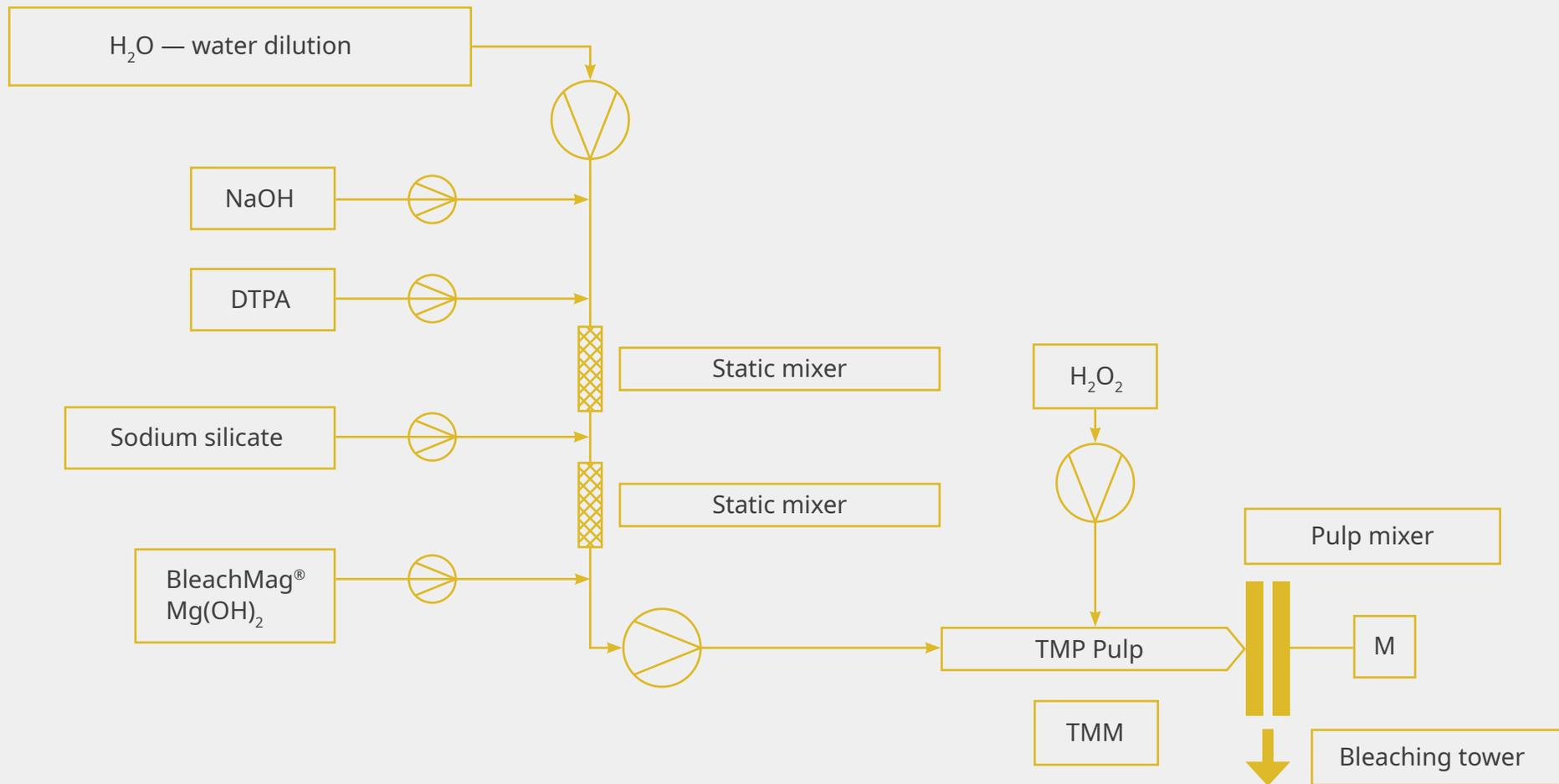
Pic. 1. Dosing scheme for BleachMag® into TMM pulp bleaching process
